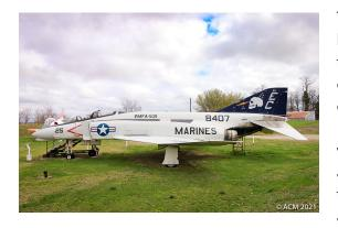
The Phantom is a large fighter with a top speed of over Mach 2.2 and can carry more than 18,000 pounds of weapons including air-to-air missiles, air-to-ground missiles, and various bombs. Beginning in 1959, it
